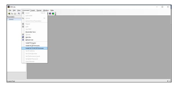
Selecting 'Install AC15/20 Firmware" will open the DCT plugin, as shown below. Clicking on the "Scan" button will start a network search for all connected AC20 products. Once the network scan is completed, any AC20 that have been found will appear, and the Ethernet settings can be edited.
