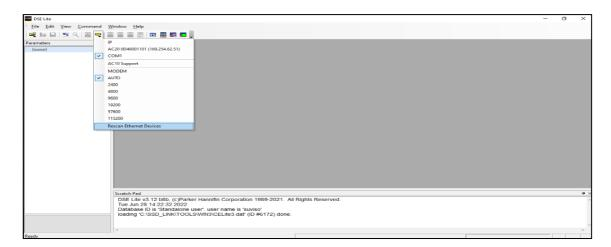
Once the network scan has been performed, any AC20 connected to the network will appear and DSE Lite can connect to the drive by selecting it from the communications settings dropdown menu as shown above.
